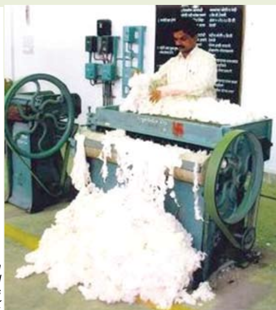
Single Roller Gin manufactured by Platt Brothers Oldham UK
