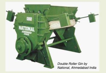
Up to the year 1970, the Double Roller Gins were manufactured using gun metal bushes as the bearings were in the developmental face and had higher friction. In 1972, all the gun metal bushes were converted to bearings which resulted in electrical power efficiency. In 1995, the working width of the Double Roller Gin was increased to 1191 mm to increase the productivity and commensurate changes were made in all other components successfully.
