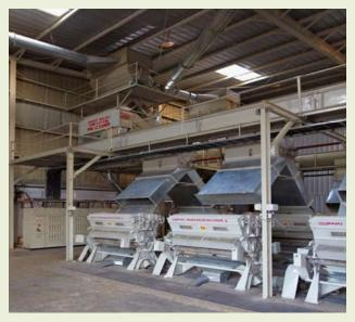
Photograph of Central Screw Conveyor Distribution System Courtesy: Bajaj Steel Industries Ltd., India.
