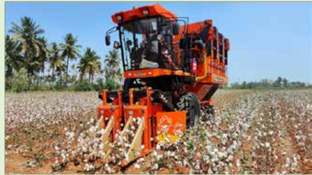
Fig.3: ICAR-CICR cotton variety Suraksha being harvested using two row spindle type cotton picker
